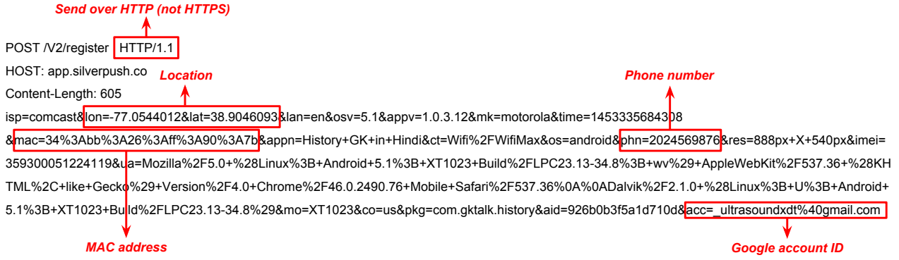
Fig. 1. An example of an insecure, non-standardized implementation of the ultrasound-enabled applications. HTTP POST request sent by an ultrasound-enabled app that we found on the Google Play Store, violating the user’s privacy and security practices: (1) The framework surreptitiously collects the user’s private information, including the Google account ID, phone number, geolocation, the device MAC address, and other information; (2) The data is sent insecurely over HTTP (instead of HTTPS).
