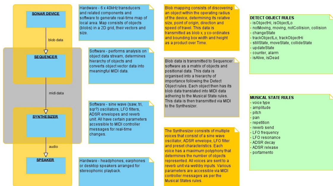
(Fig. 10: image: concept diagram – EarFreq-rev2.0.jpg)
